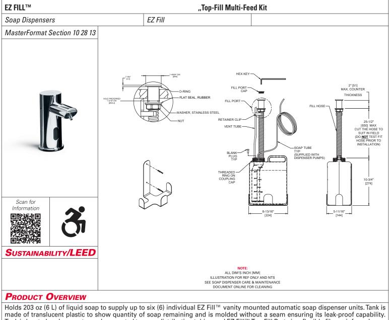
Tank is located under counter and connected to soap distribution tubing and EZ Fill<sup>TM</sup> Top-Fill Port via a flexible fiber-reinforced soap fill hose. EZ Fill™ Top-Fill Port and cover are made of highly polished chrome plated brass (for matte black finish use suffix -41). Includes: 6 Liter Container, Top Fill Tube, Counter Fill Port with Cover. KIT ONLY, DISPENSER NOT INCLUDED
